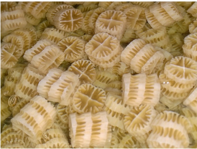
Clewer R-4000 bioreactor and carrier elements with biofilm.
